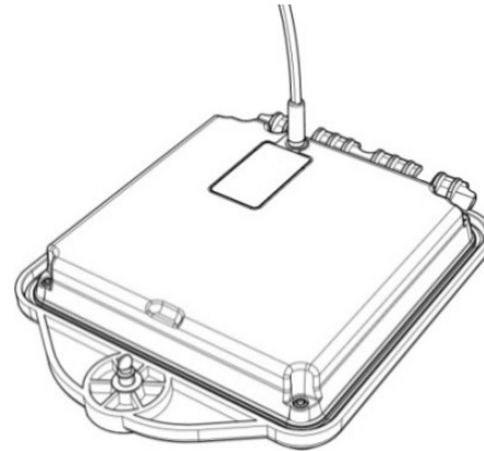
Figure 4.13 Charging the transmitter Li-Ion battery pack
