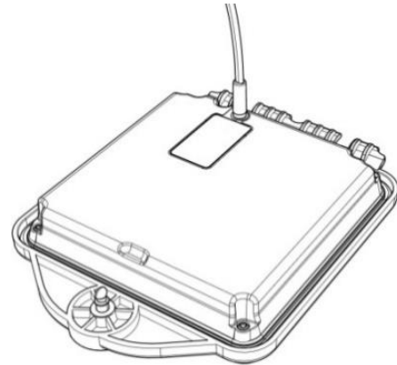
Figure 4.13 Charging the transmitter Li-Ion battery pack
